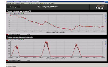
Temperature and light monitoring, used to calculate energy consumption costs
